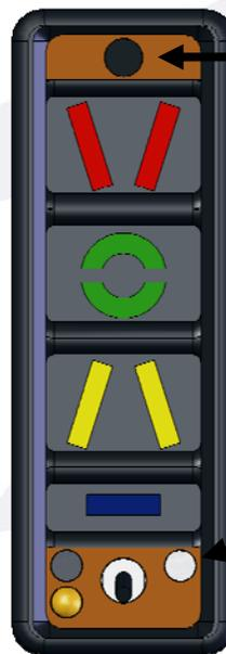
Cover Photo Cell here to simulate "DARK" setting or shine light to simulate "DAYTIME" setting.
